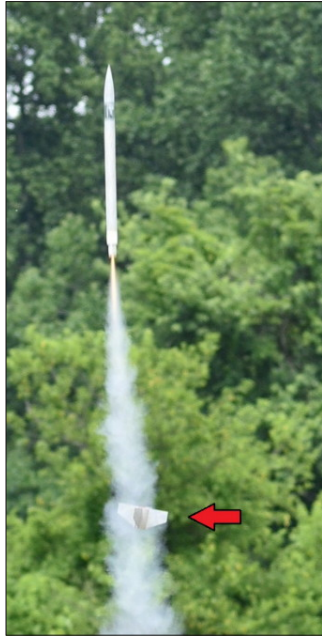
The fin unit (arrow) separated in-flight during the launch of the Marine Corps payload model. Credit: Alex Mankevich
