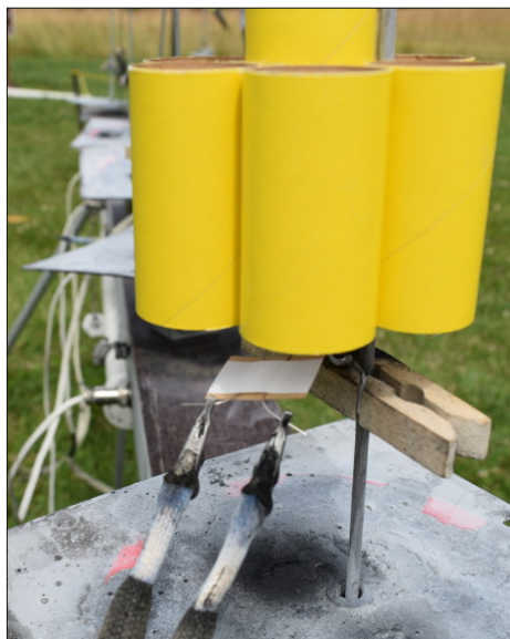
Square metal blast deflectors will turn sooty with motor exhaust after several rounds of launches. Credit: Alex Mankevich
