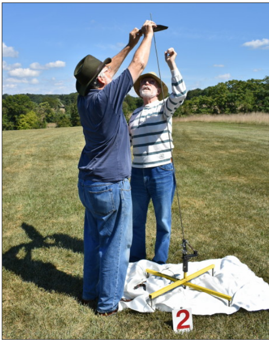
A Fire Blanket (100% woven glass fabric) protected the grass under the pad as James Miers (L) and Brian Beard (R) placed the blast deflector down the 1/4 inch launch rod. Credit: Alex Mankevich
