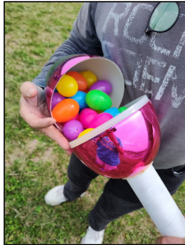
A close-up of the eggs-holder capsule for Chris Greco's egg loftor rocket. Sadly, this model did not fly due to stability issues. Credit: Sarah Jackson
