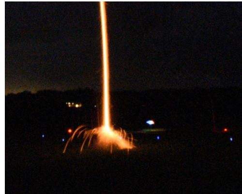
This image from the 2018 John McCoy Night Launch illustrates the cascade of glowing, partially burnt material that bounces off the metal blast deflectors. Credit: Alex Mankevich
