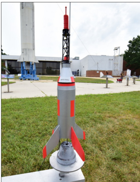
Clay pots have been used for several years in conjunction with metal blast deflectors to protect the Goddard launch rack. Credit: Alex Mankevich
