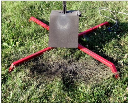
The leading edge of this blast deflector was not angled upwards - causing the grass to become scorched. Credit: John McCoy
