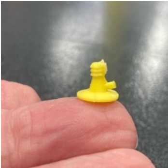
A magnified view of the extraneous plastic appendage found on the yellow standard engine igniter plugs. Credit: Michael Cochran
