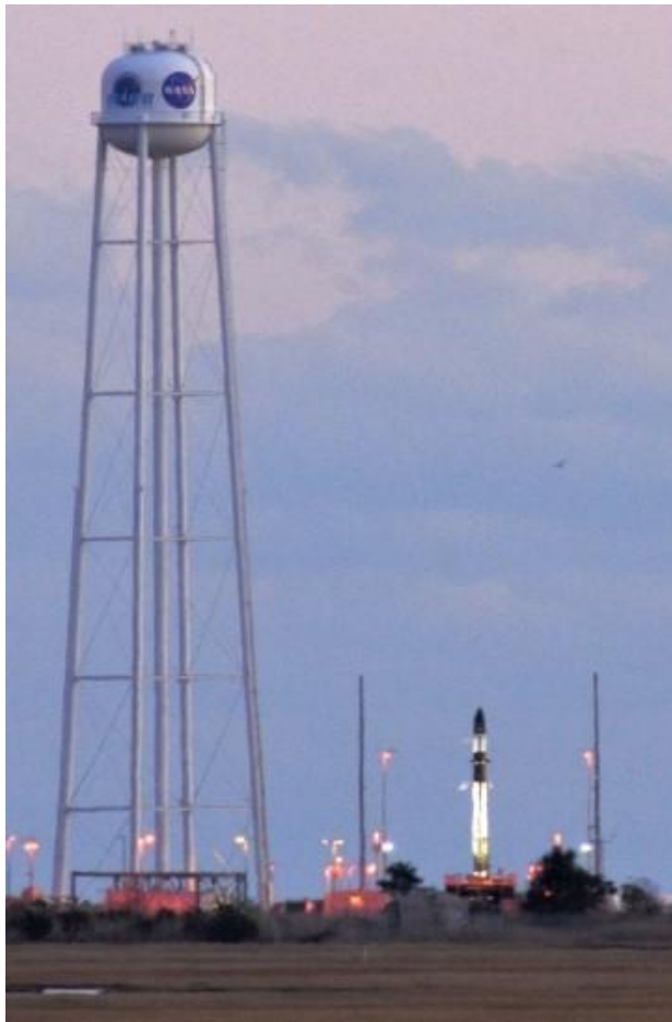
Above: The nearly 60 feet tall Electron rocket stands about one-third the height of the water tower. Portions of the normally black colored rocket body turn white due to frost as the supercooled propellants are loaded. Photo: Alex Mankevich
