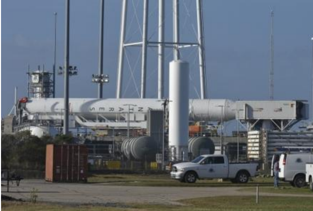
Left: The rectangular Mobile Clean Room (MCR) is attached to the horizontal Antares 230+ rocket's fairing at the right side of this image. The MCR is used as a clean and temperature-controlled environment in which to perform a final load of time-critical cargo at twenty-four hours before lift-off. The top of the fairing pops off and technicians can access the pressurized cargo module of the Cygnus spacecraft. After the final load is completed the Antares rocket is rotated back to vertical on the launch pad.
