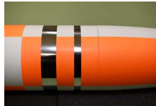
Left: Instrumentation Section Bands applied.
