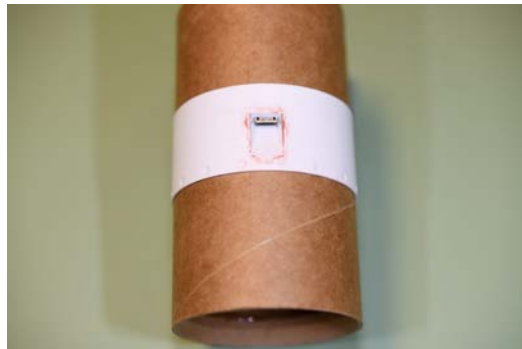
Left: Umbilical Port Installed
