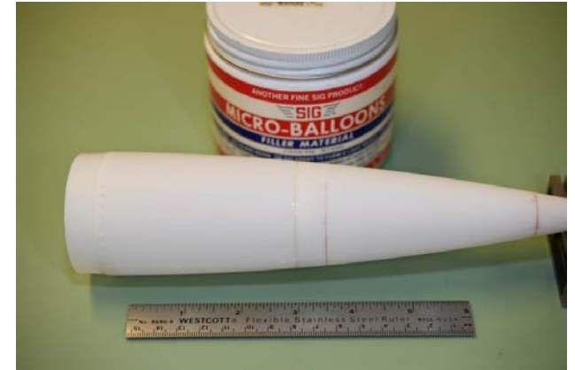
Above: Filled Joint
